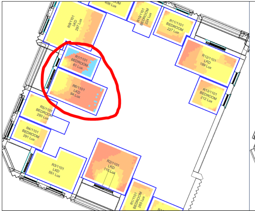
Figure 21 – Internal layout and poor daylight to Block A.
